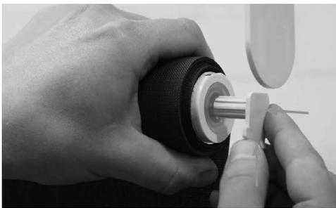
3. Put the limiter clip back in its place in a vertical position.
